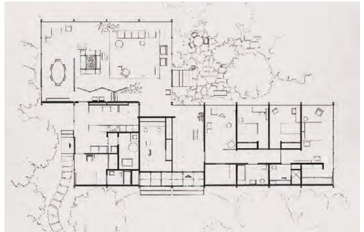
Floor plan showing front hall and Ben Rose's studio, living, dining room, bedroom wing, and service area
