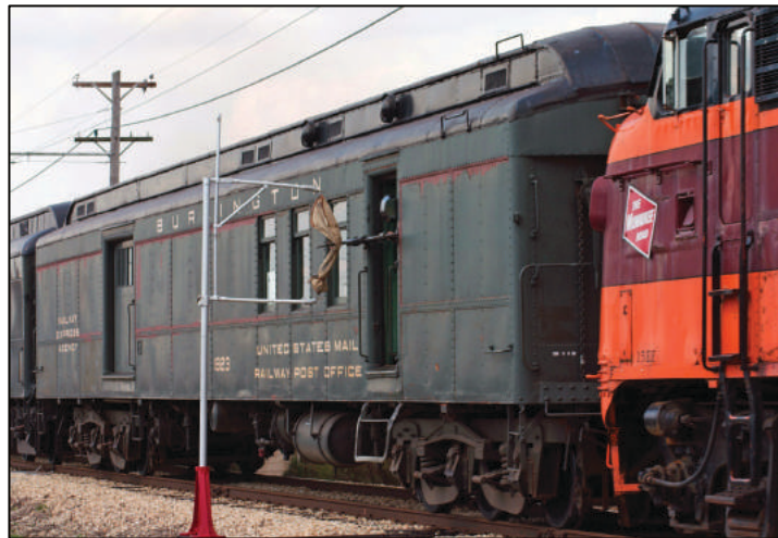
This is the moment a Milwaukee Line mail car snatches a mail pouch from a mail crane while in motion.
